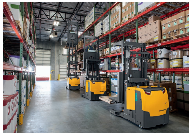
Toromont Material Handling provides specialized equipment such as this electric powered Jungheinrich Class II reach truck that is specified to perform in the narrow confines of warehouses and logistics centres.
