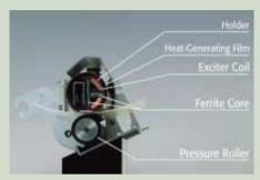
Canon's originally developed color IH fixing technology radically reduces warm-up time.
