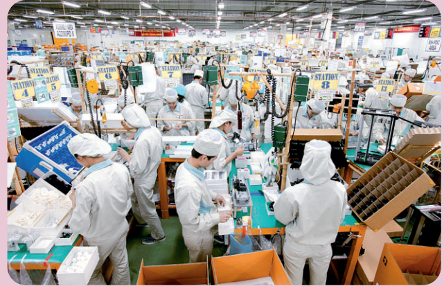
The cell production environment employed at Canon's factory in Vietnam draws on the strong traditions of Vietnamese craftsmanship not only for achieving high production standards, but also for making some production equipment.
