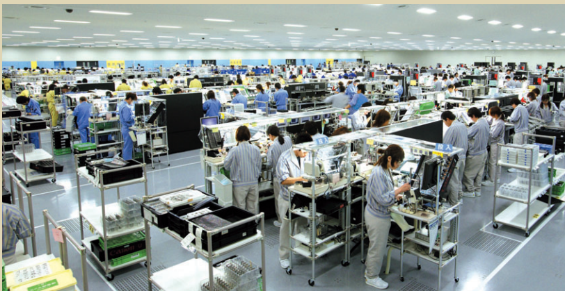
The absence of internal pillar supports makes flexible cell production system layouts possible at the new plant at Oita Canon, Inc.
