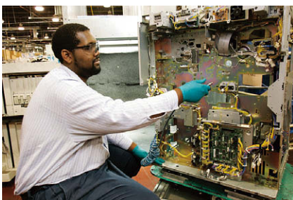
Used copiers disassembled, cleaned, reassembled and remarketed in almost new condition
