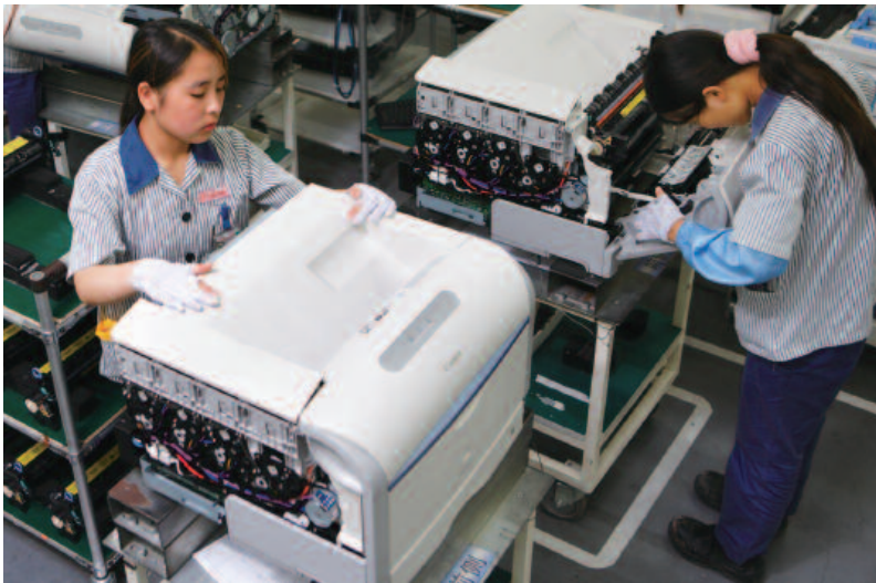
Producing color LBPs and copying machines through the cell production system at Canon (Suzhou) Inc. in China
