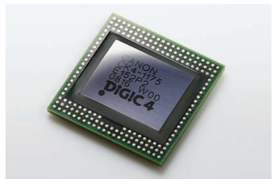
DIGIC 4 imaging processor offers exceptionally fast signal processing for Canon's digital cameras.
