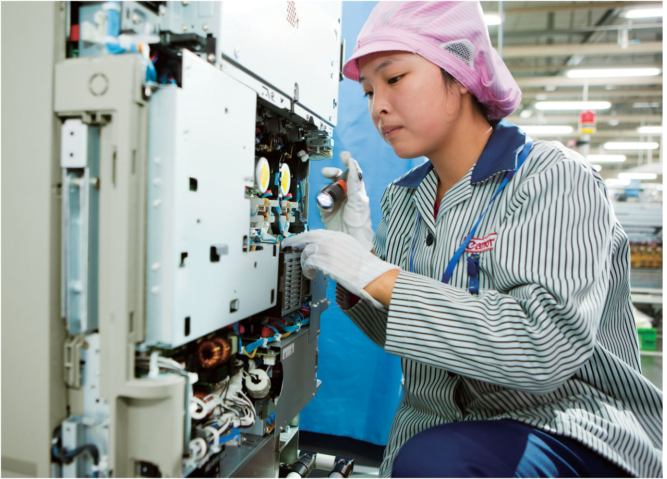
In China, Canon (Suzhou) Inc. conducts cell production of imageRUNNER ADVANCE models.
