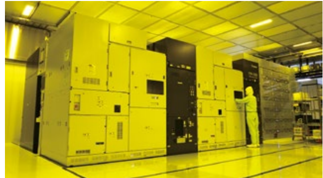
Mass production verification of nanoimprint manufacturing equipment is underway at Kioxia's Yokkaichi plant. (Japan)
