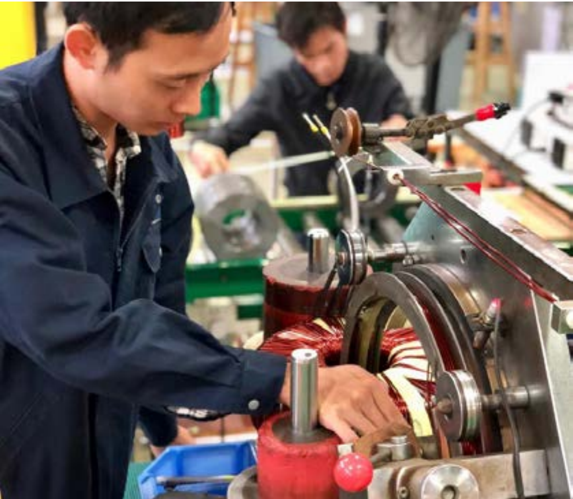
Pictured: Opposite page: Board visits the Noratel factory in Foshan, China. Above, clockwise from top: copper winding onto a toroidal transformer used in medical applications; semi-finished goods testing, prior to the next stage of manufacturing; and connecting cable sensors onto an integrated transformer and reactor assembly used in transportation applications.
