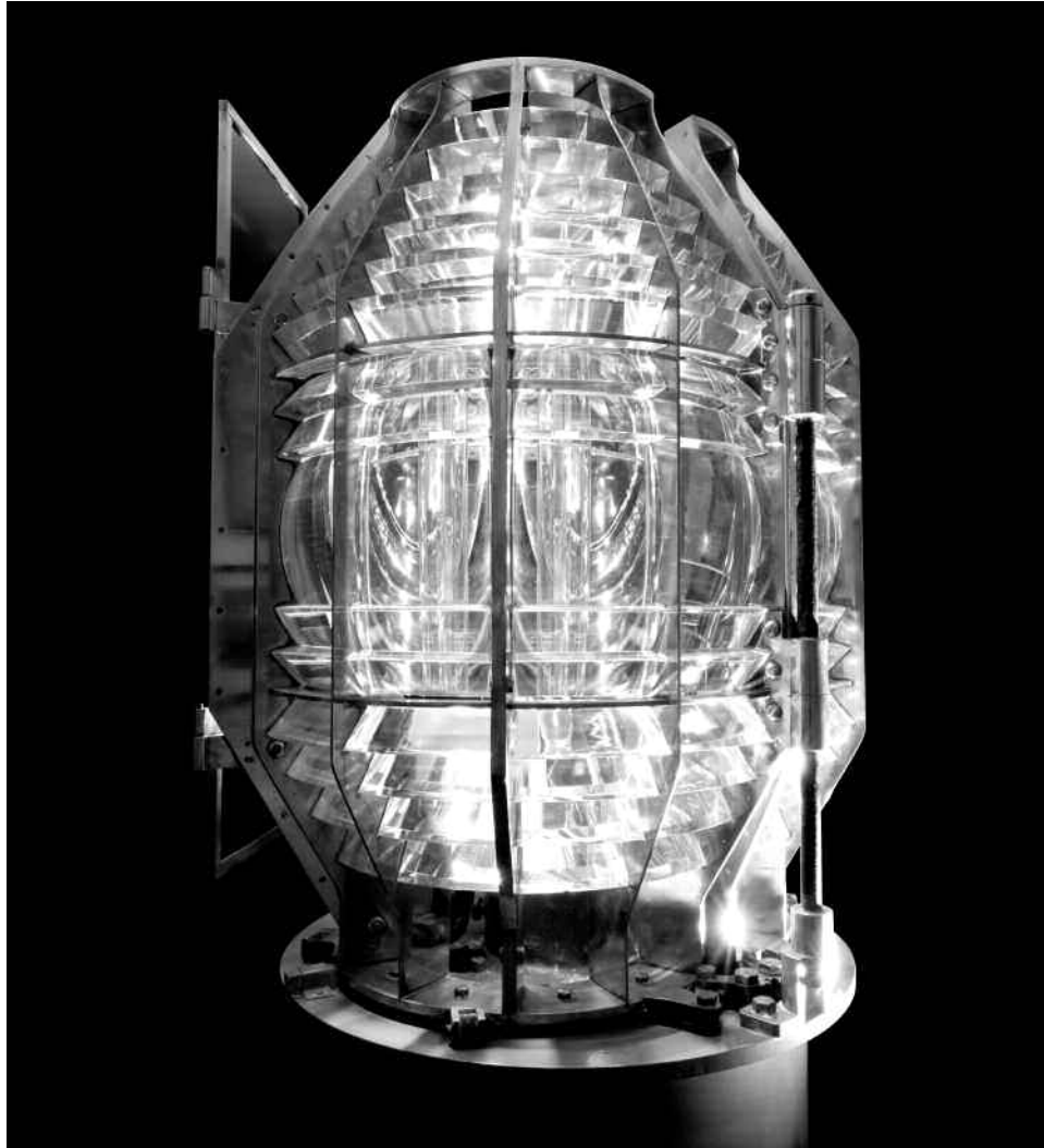
The original Fresnel lens from the Watch Hill Lighthouse. The lens features beautiful cut glass prisms, set in brass frames, that collected and concentrated light emitted from a 1000-watt bulb and directed it out along horizontal beams.
