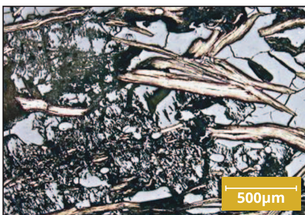
Figure 9. Photomicrograph of coarse graphite flakes (in white) from Siv004 (56m to 57m)
