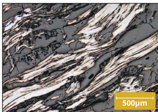
Figure 10. Photomicrograph of graphite flakes (in white) from Siv001 (73m to 74m)
