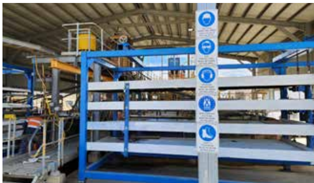
Eight additional shaker tables have been installed and commissioned to increase processing capacity.
