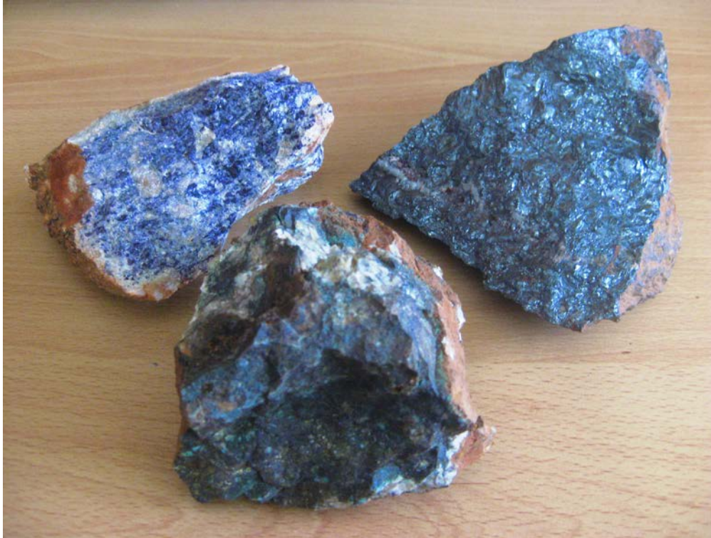
Figure: Fluorite, Massive Haematite and oxidized Chalcopyrite samples from the Illogwa Project
