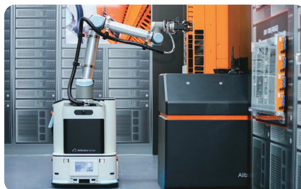
▲ Alibaba Cloud's inspection robot Tianxun is equipped with controllable arm to increase the maintenance efficiency of data centers.
