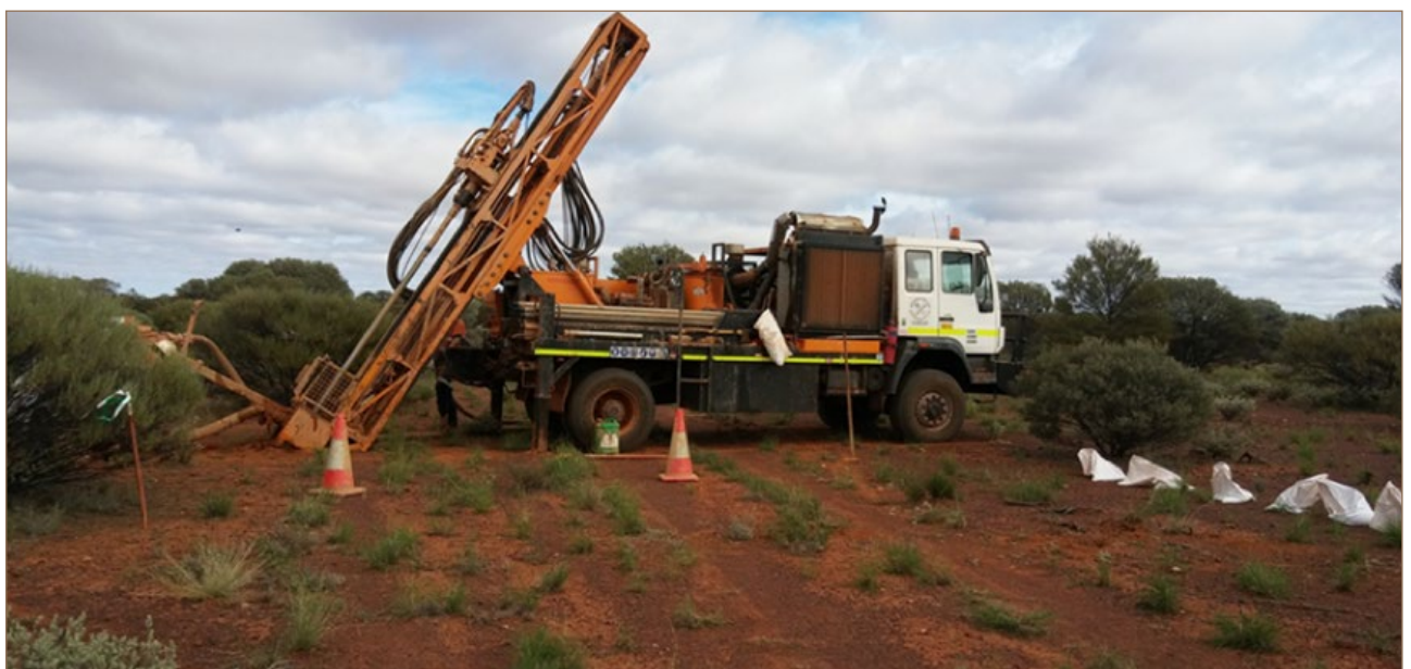
Aircore Drill Rig at Indomitable East
