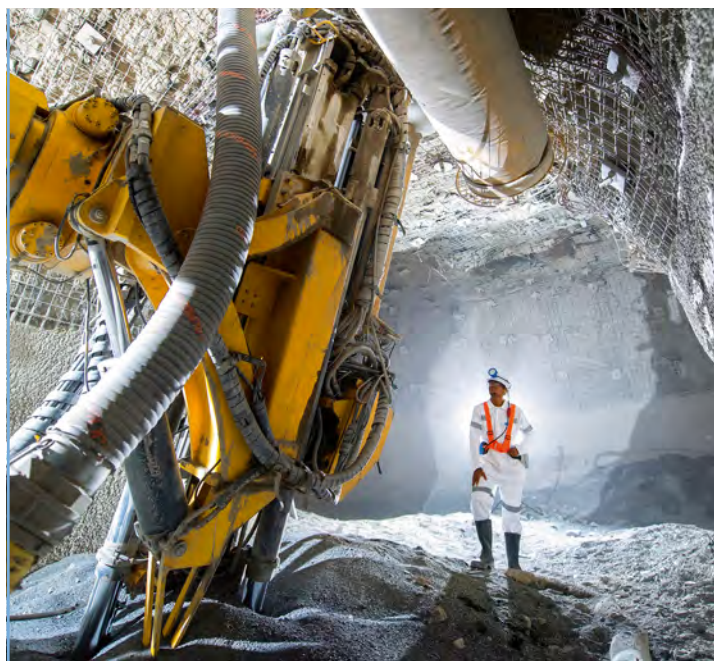
A Simba ME&C (Epiroc) production drill-rig used for drilling long hole blast rings in the SLC at Finsch.
