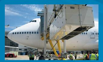
JBT AeroTech PCA units are reducing operating costs and carbon impact for a growing number of air transportation customers. Our point-of-use pre-conditioned air (PCA) units enable jets to turn off their engines at the gate, reducing fuel consumption, noise and carbon pollution, and, because most units are bridge mounted, ramp congestion.
