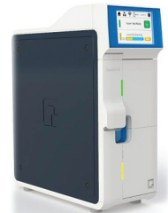
Savanna , currently in development, sample-to-answer molecular system that can run both real-time PCR and isothermal helicase-dependent amplification assays.
