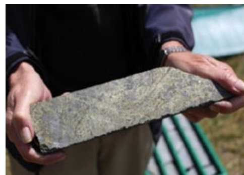
Figure 2: A section of core from CH-DDH012 from approx. 190m running 1.8% Cu, 0.8g/t Au, 123g/t Ag
