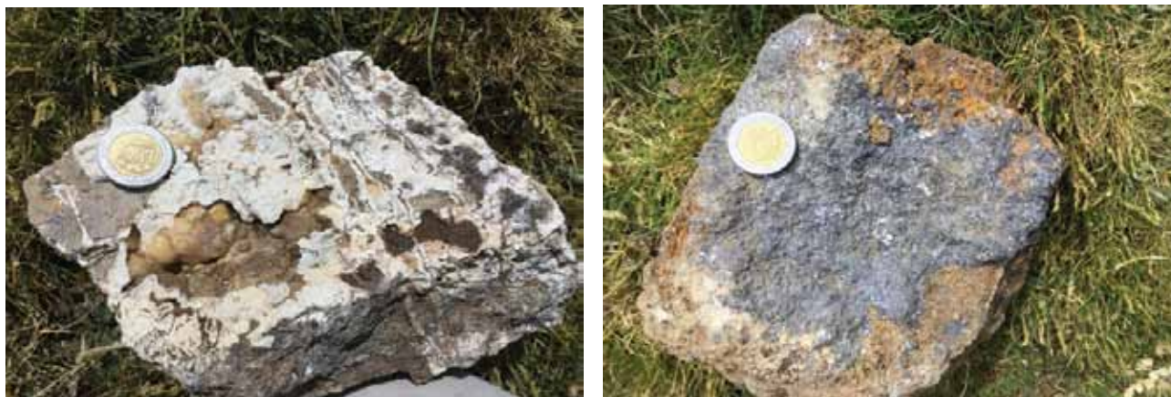
Figure 5 ABOVE LEFT: Vein material from an old mine working at Cerro Rayas. This sample returned 32.07% Zn, 349g/t Ag and 20.19% Pb. ABOVE RIGHT: More weathered vein material from the same working that returned 41.59% Zn.
