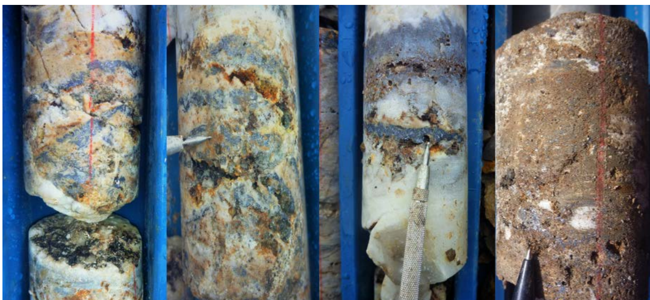
Figure 3: Examples of mineralised veins identified in holes RDDH-001 and RDDH-002. A, B, C Galena and smithsonite within calcite-barite gangue material in vein HV-09; D Fe-oxides with relic galena in vein HV-06; E Veinlets of galena with calcite-barite concordant with bedding and cross-cutting bedding in a new vein.
