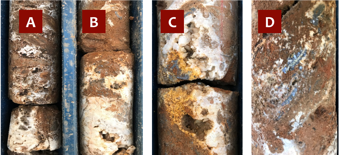
Figure 4: Examples of mineralised veins and mantos identified in holes RDDH-004 and RDDH-011. A, B Highly gossanous manto with relic galena and calcite-barite gangue; C, D Highly gossanous vein with relic galena and calcite-barite gangue. Where weathering is particularly well-developed sphalerite is generally missing and smithsonite is also partially or completely dissolved.
