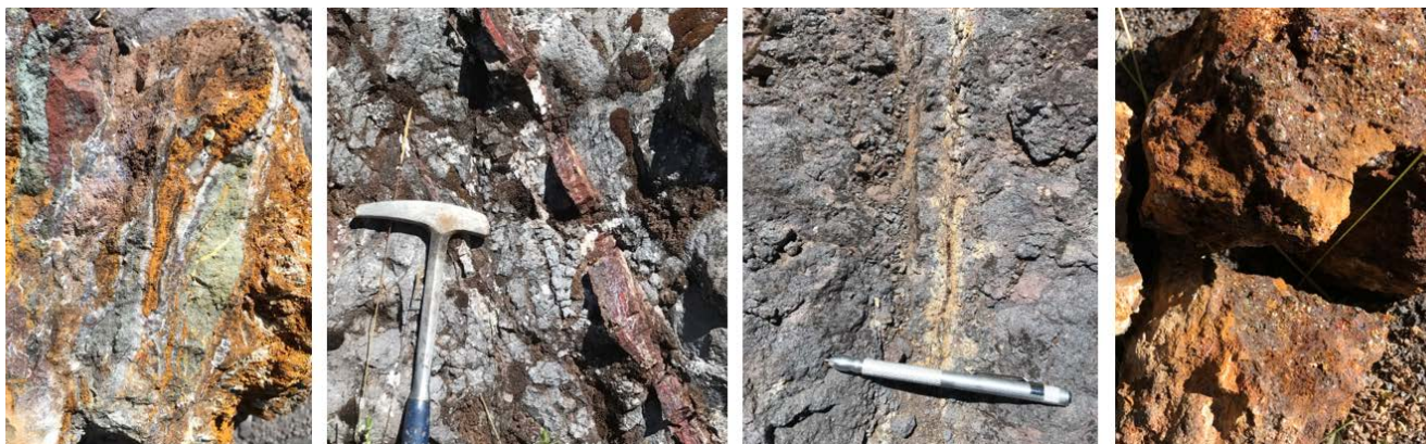
Figure 7: Various outcrops at Colina Roja showing strong epithermal alteration, veining and sulphide-gossan development. The far-right photo shows a strongly gossanous-sulphide bearing vein that hosts 3.75% Zn, 136g/t Ag and 3.13% Pb.
