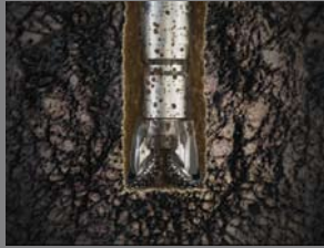
The drilling process generates chips of rock known as cuttings.
