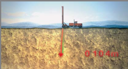
A 2 degree deviation at the surface can lead to a 35 metre lateral displacement at a hole depth of 1000 metres.
