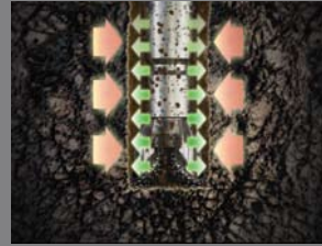
Fluids stabilise and keep the bore hole open.
