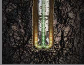
Fluid is pumped down the drill pipe lubricating the drill bit and returning cuttings to the surface.
