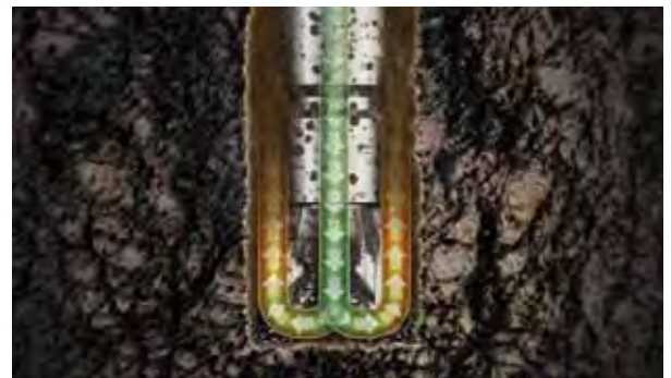
Fluid is pumped down the drill pipe lubricating the drill bit and returning cuttings to the surface.
