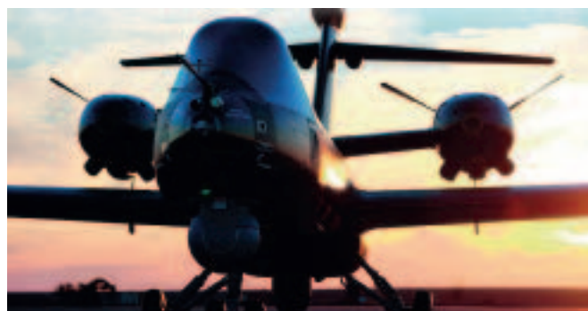
Mantis – The next generation autonomous system, Mantis, completed its maiden flight in Woomera, South Australia, in October. Mantis, an advanced technology demonstrator medium-altitude long-endurance UAS, went from concept to flight in just 19 months.
