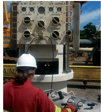
20" vertical integral collet connector for offshore Brazil.
