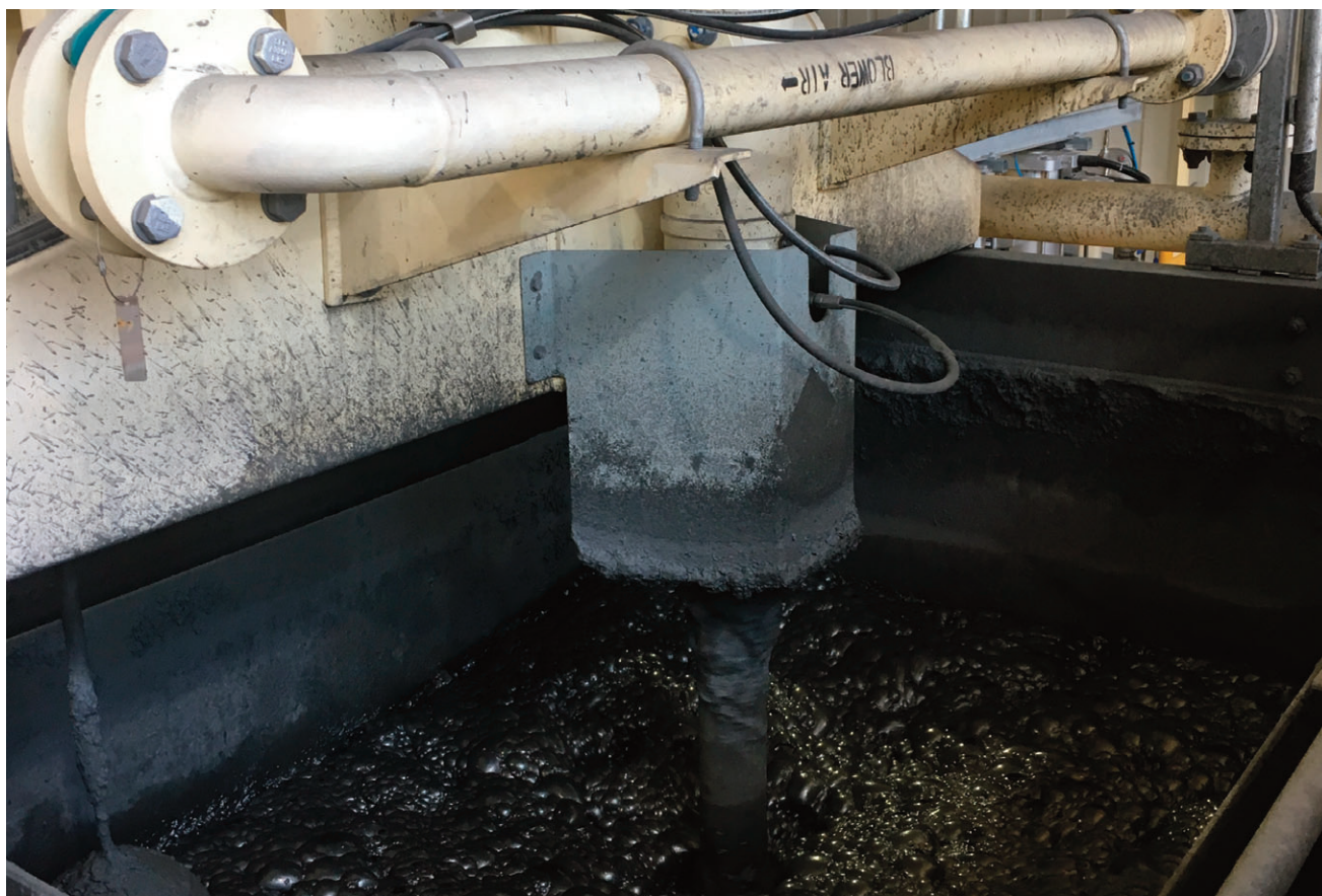
Figure 6: IsaMill™ undergoing an internal inspection.
