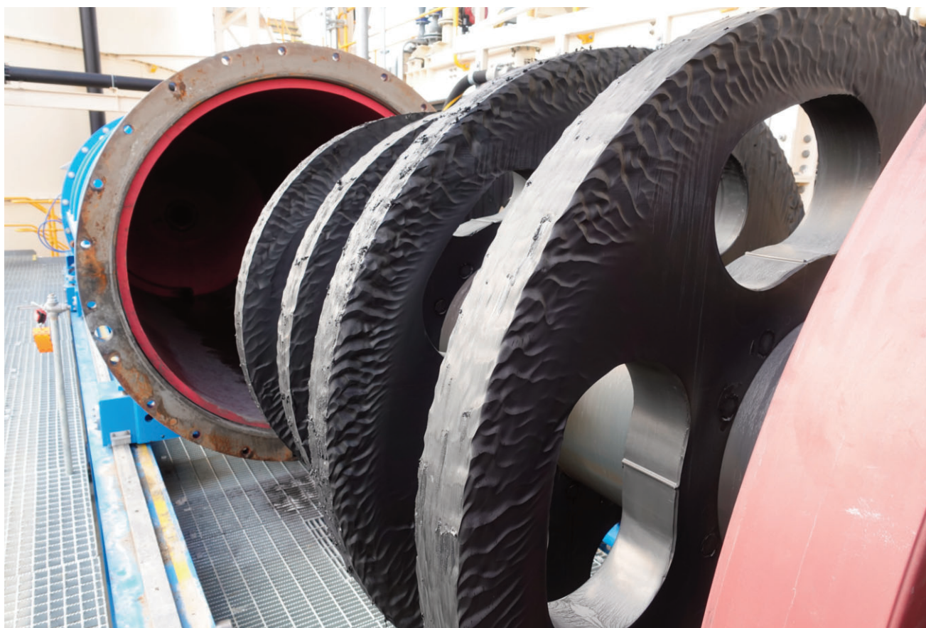
Figure 6: IsaMill™ undergoing an internal inspection.
