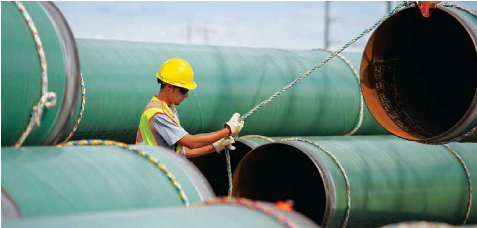
Bredero Shaw's facilities in Camrose, Alberta and Regina, Saskatchewan provided fusion bond epoxy anticorrosion coatings for the Keystone XL Project.
