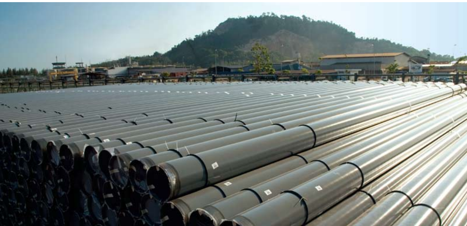
Bredero Shaw's facilities in Australia and Malaysia provided anticorrosion and flow efficiency coatings for the 945 km Epic Energy QSN3 Project.
