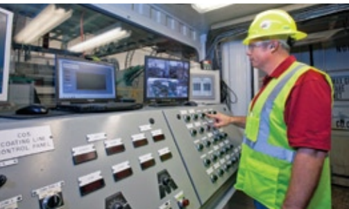
All control systems are built into Brigden's modular design, which eliminates the need for time-consuming installation of lighting, electronics and plumbing on site. As a result, this full-service coating plant can be mobilized and into production in six weeks.
