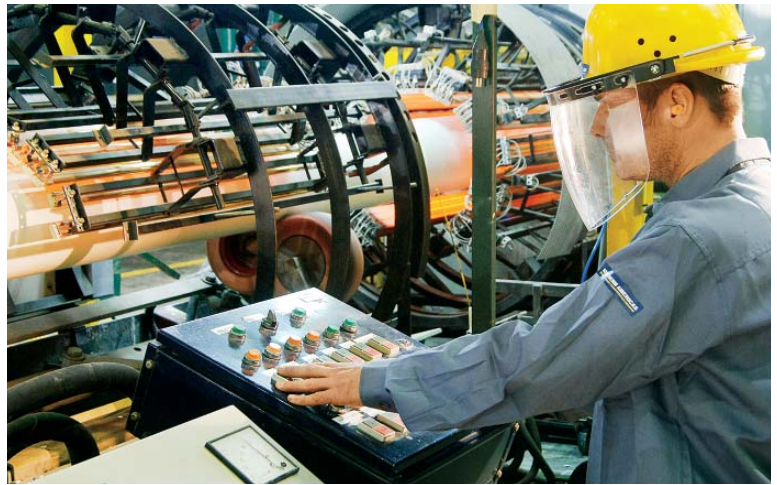
Top: Socotherm's advanced Wetsokote® thermal insulation coating system undergoes infrared heating.
