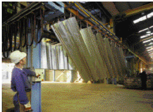
Part of the UK's first fully automated hot-dip galvanising plant at Birtley.
