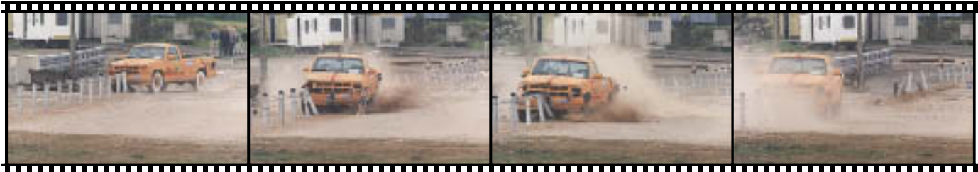
Sequence showing testing of the Brifen wire rope system for the US market
