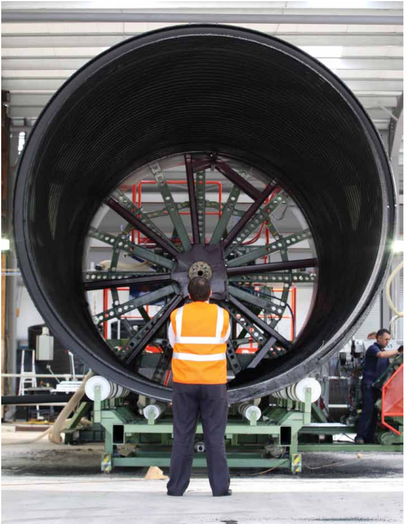
Asset Weholite HDPE production line manufacturing the largest plastic pipe in the world (3.5m diameter) for the AMP5 market.
