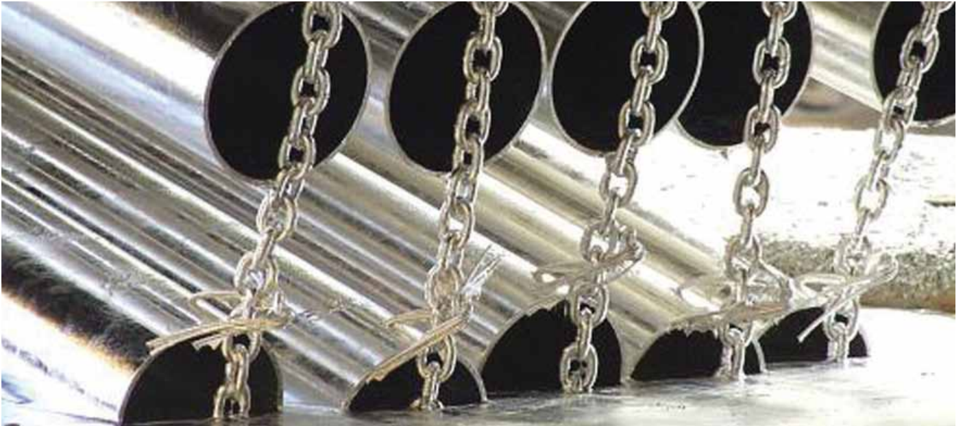
Steel piping being galvanized at a Joseph Ash UK galvanizing plant.
