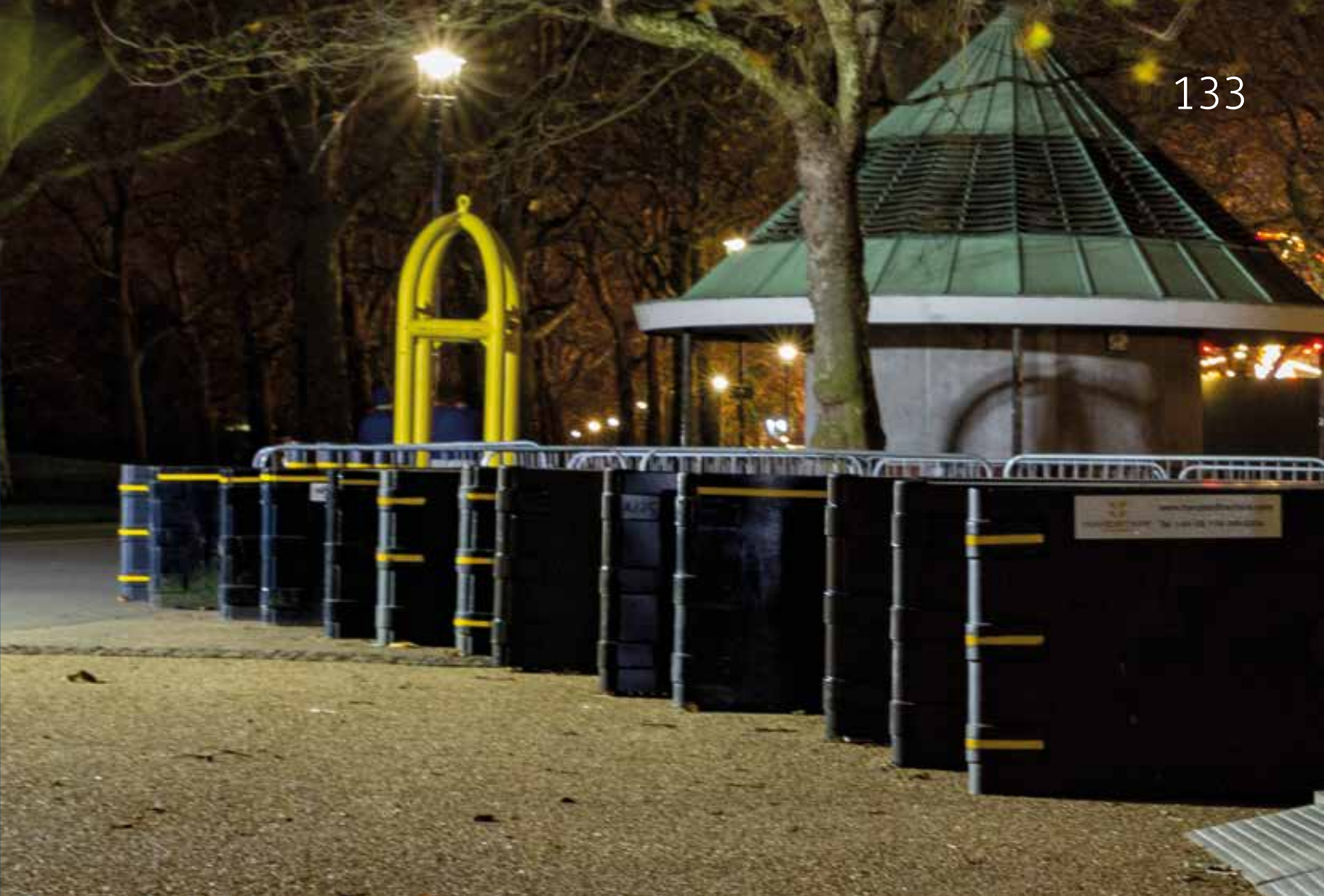
Top: Hostile Vehicle Mitigation barges in Hyde Park London – Keeping Pedestrians Safe
