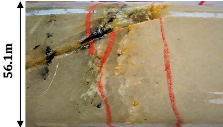
Figure 11: Visible gold in diamond core from ZDD1440 – reported 184.55 g/t Au over 0.55m from 61.8m.
