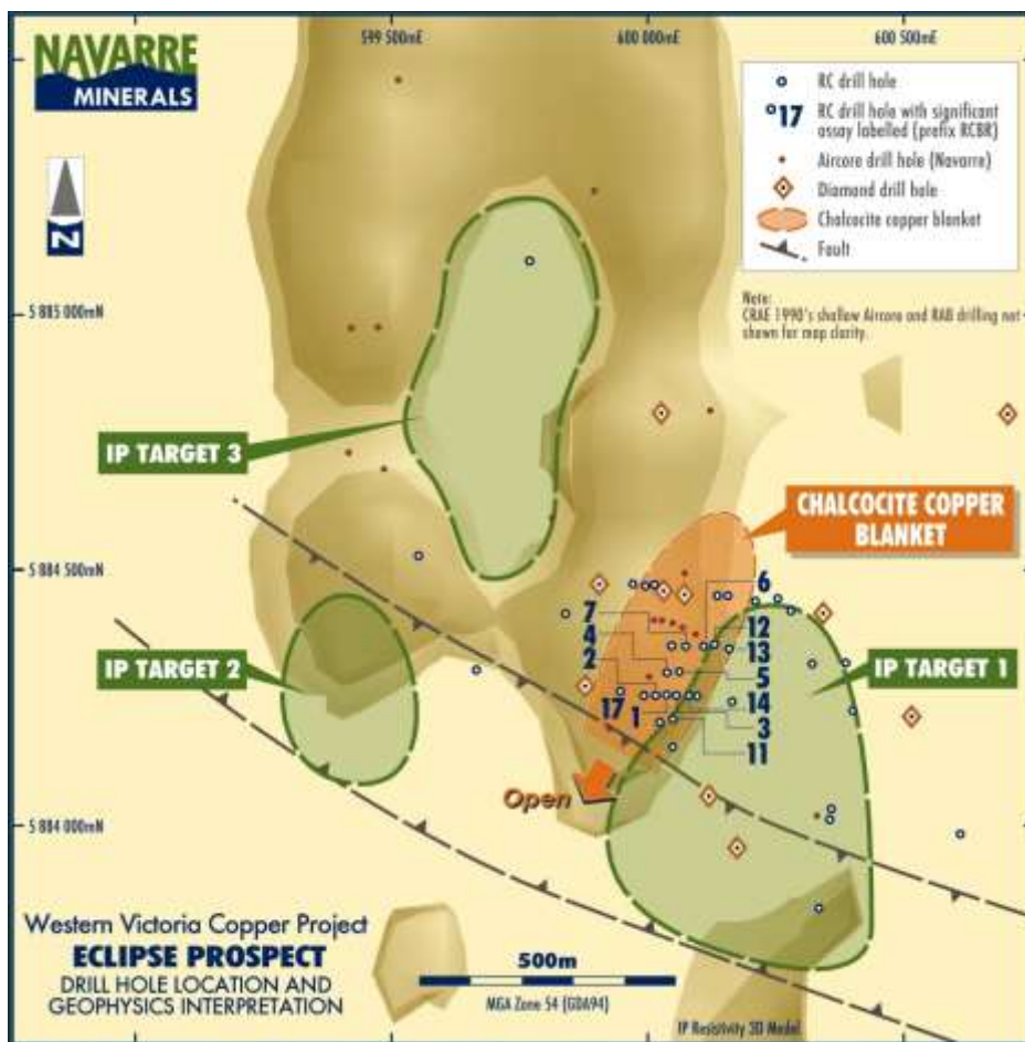
Figure 2: Plan view of the Eclipse prospect showing location of three IP geophysics targets, location of the recent RC drill program and outline of known chalcocite copper blanket.
