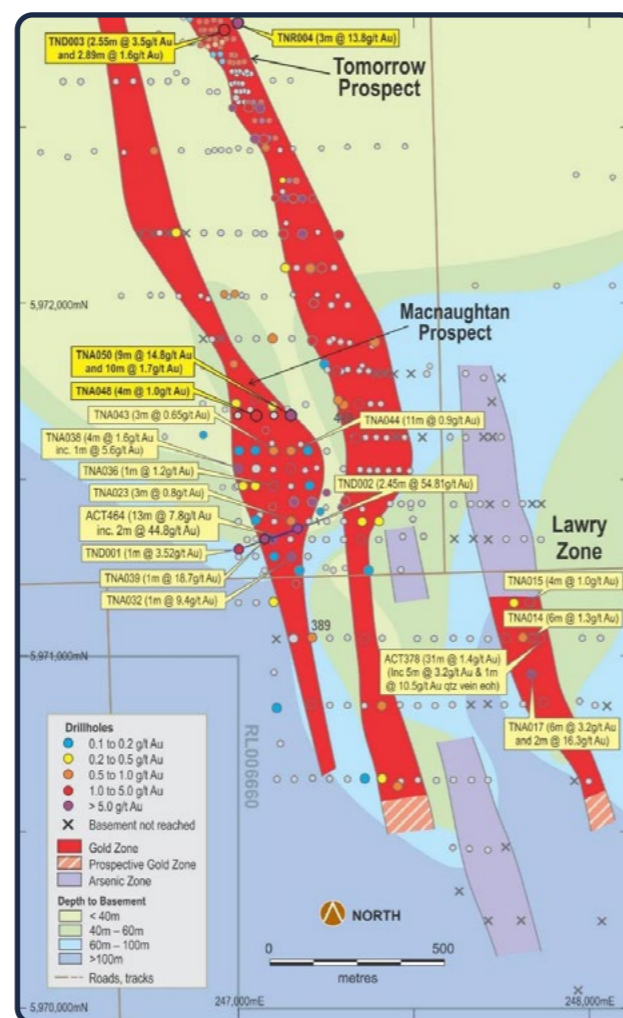
Figure 9: Plan of the Macnaughtan, Tomorrow and Lawry prospects showing significant 2021 drilling results. (Diagrams reproduced courtesy of Catalyst Metals Limited).
