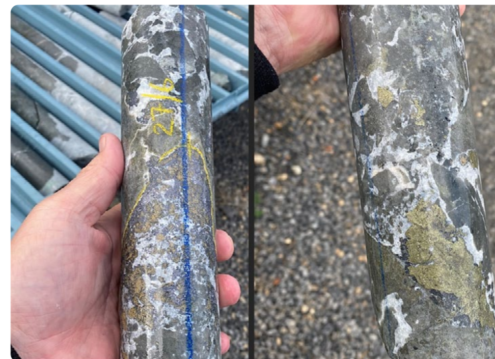
Figure 7: Straw-yellow sphalerite (zinc) and grey galena (lead) mineralisation at 213m in GDD003 (LHS) and chalcopyrite (copper) mineralisation at approximately 215m down hole in GDD003 (RHS).
