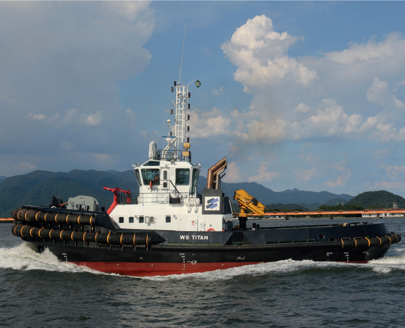
The tugboat WS Titan was built at the Group's shipyard in Guarujá, São Paulo in 2015. With 80 tons bollard pull the WS Titan is the most powerful tugboat currently operating in Brazil.
