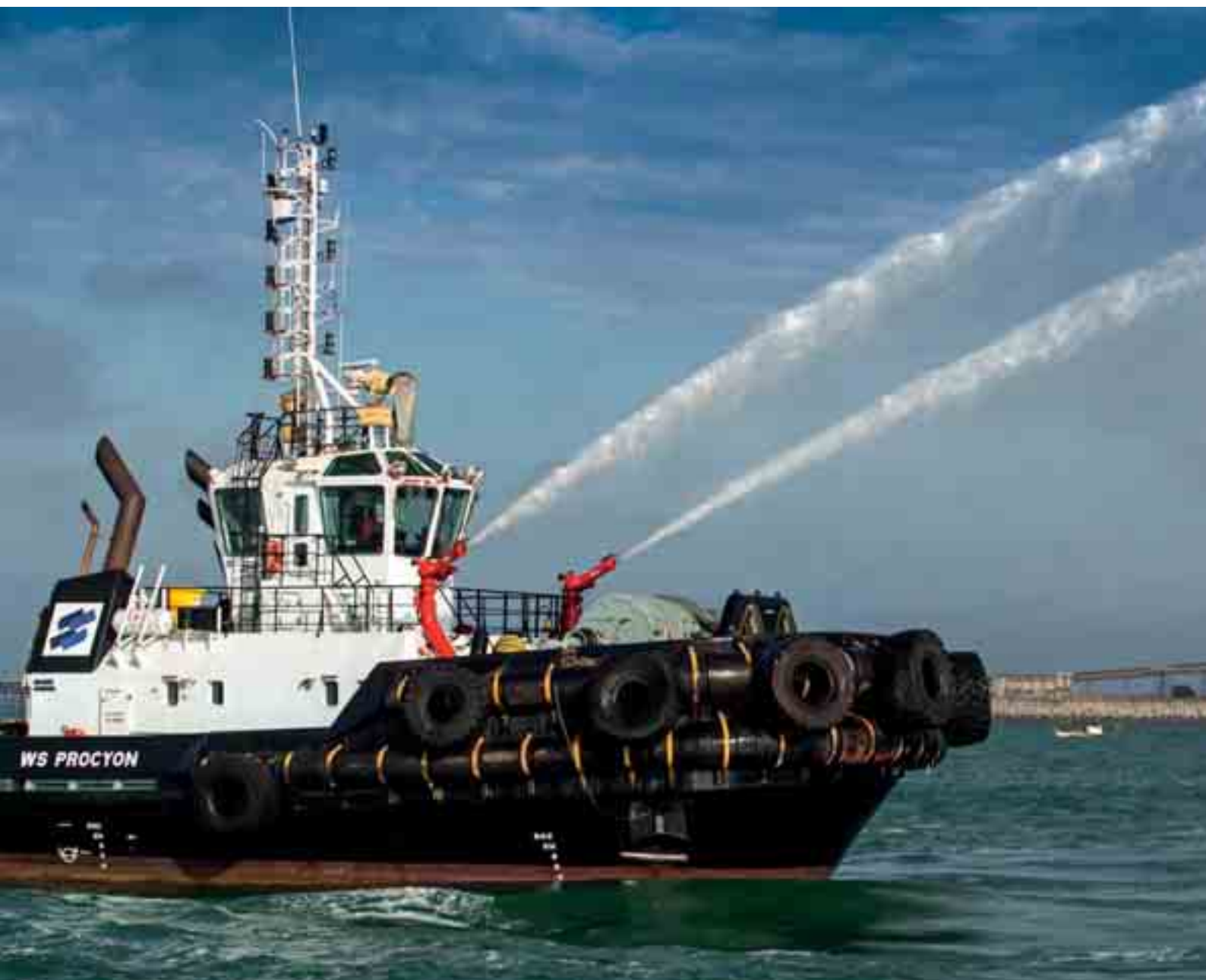
The tugboat Procyon built at our shipyard in Guaruja is equipped for external firefighting enabling it to tackle fires on other vessels or waterfront property.
