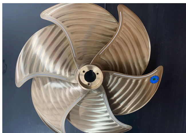
Figure 14: First ever 48" diameter VEEMSUPERYACHT series 6 blade propeller with patented Interceptor strips
