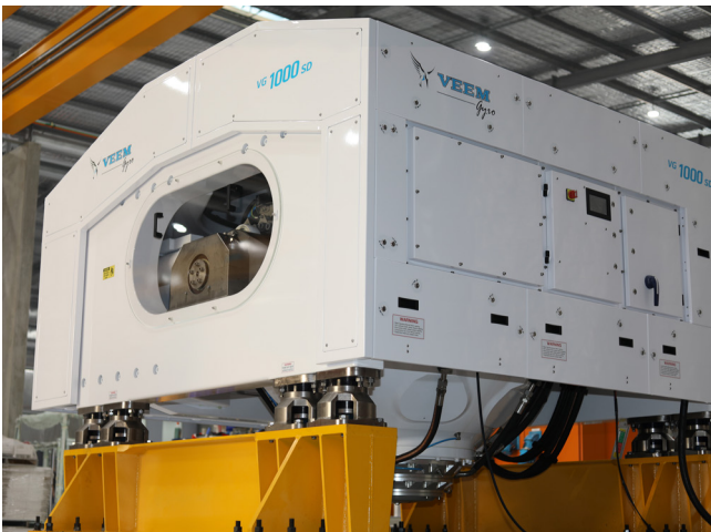
Figure 3: The most powerful marine gyrostabilizer in the world. VEEM'S VG1000SD is suitable for large Super Yachts, commercial workboats and defence vessels
