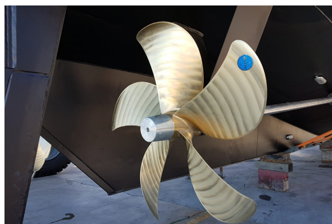
Figure 11: A new installation of a VEEM Marine VEEMStar 5-blade propeller in Italy
