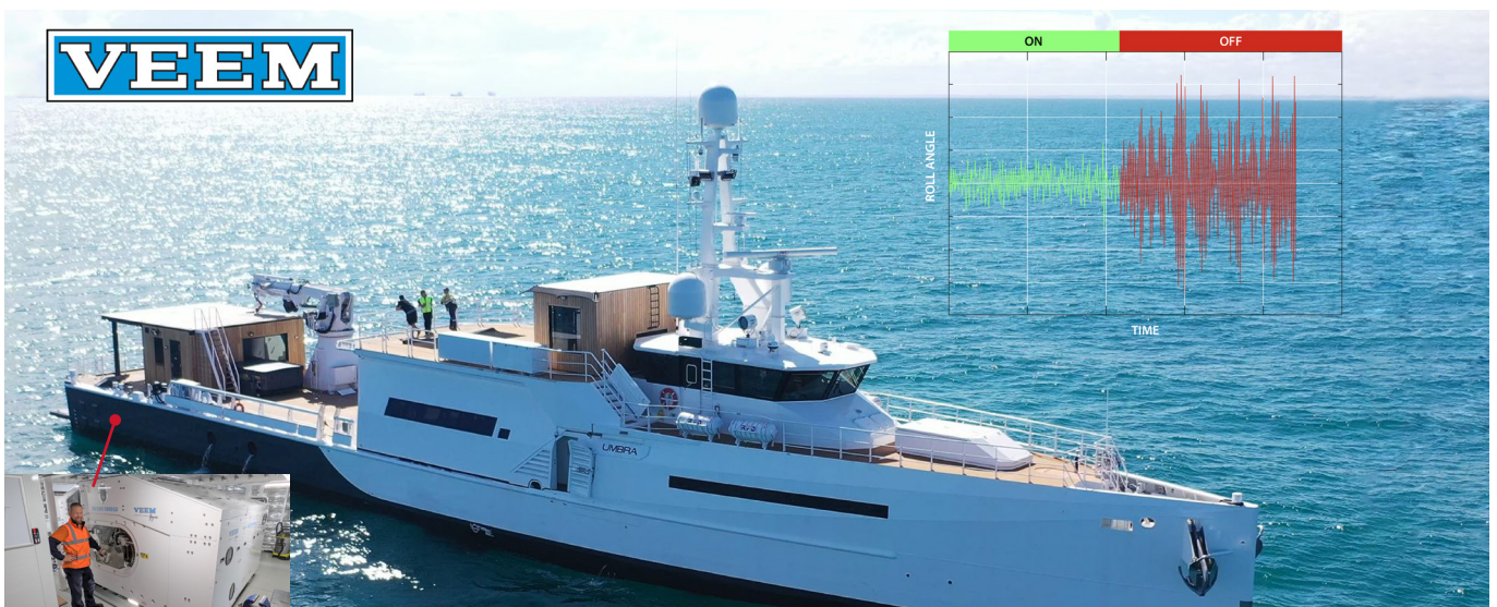
Figure 1: MV Umbra, a 60m Damen YS5009 exploration vessel, carried out successful sea trials off Fremantle, WA, after a VEEM Marine VG520SD gyrostabilizer was installed.
