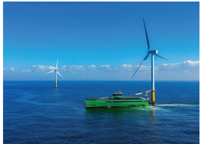
Figures 1 & 2: The Damen FCS 7011 vessel "Aqua Helix", featuring the VEEM Marine VG520SD gyrostabilizer, won the Offshore Energy Vessel of the Year award in June 2022. This revolutionary "walk to work" vessel is capable of continuously sailing at speeds of up to 40 knots to enable short transit times.
