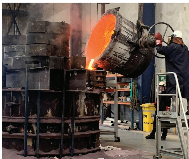
Figure 10: Pouring metal for a large casting at VEEM in Canning Vale, Western Australia.
