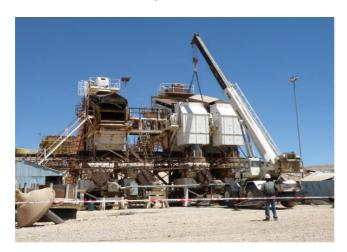
Refurbishment of critical components of the crushing and gold recovery facilities has taken place offsite and this equipment is now reassembled and recommissioned.
