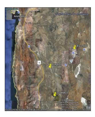
Guanaco is located in the Palaeocene/Eocene belt, a structural trend which runs north/south down the centre of Chile. This trend accommodates several large copper/gold mining operations including Zaldivar, El Peñon and Escondida.
