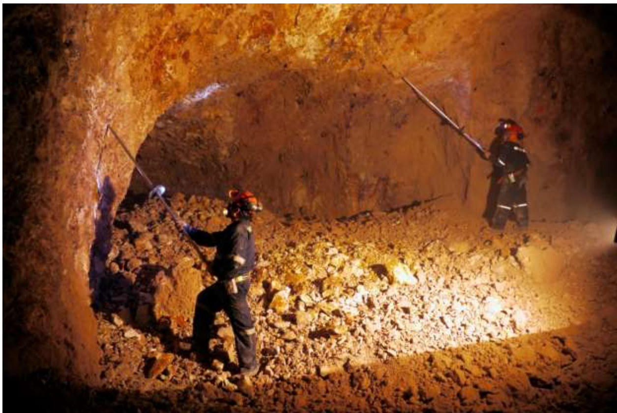
View from Cachinalito underground mine. Two miners working on scaling activity
