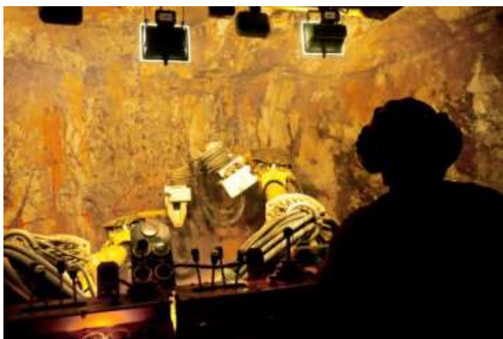
Jumbo blast drilling operation in Cachinalito underground mine.
