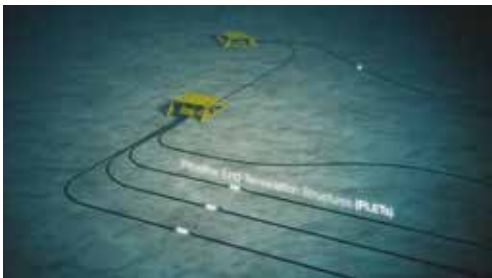
The pipeline end termination structures are utilised to connect the rigid flowlines to the risers at the FPSO and the manifolds at the wells.
