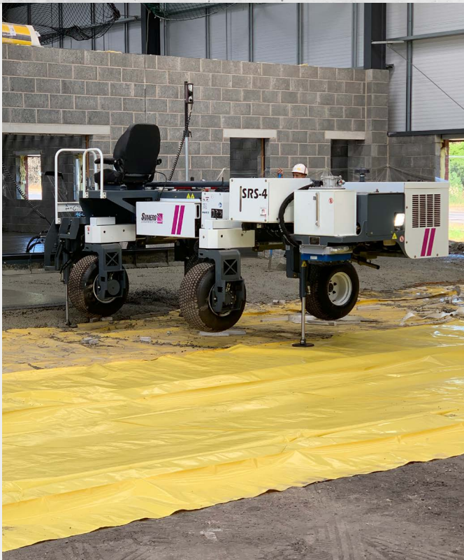
↑ SRS-4 Boom Laser Screed® in action
