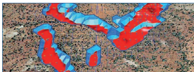
Figure 9. Waite Kauri Resource (0.8%Ni cut-off) within the optimum pit.
