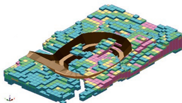
Figure 3. Showing Hepi starter pit with an ore block model- approved and ready to mine.
