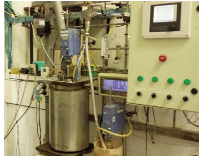
Figure 6 - Above Single Reactor Batch/Continuous Solution Neutralisation/Fe Removal Test Rig
