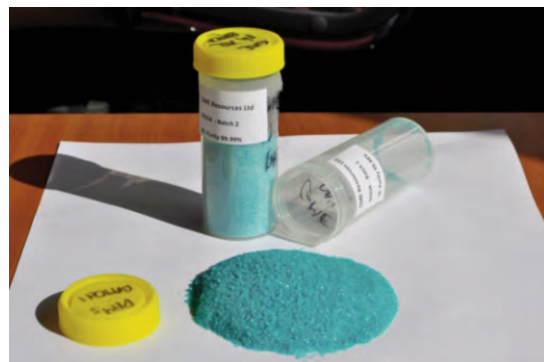
Photo above: High purity (+99.98%) Nickel sulphate products produced from the continuous pilot plant.
