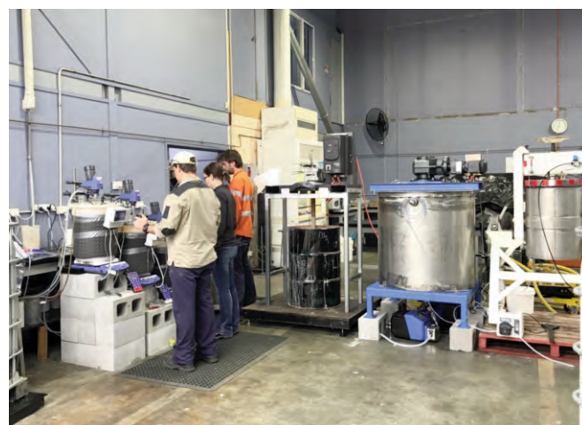
Figure 3: Pilot Plant – Solution Neutralisation Fe/Al removal tanks (bottom left) including thickener and filter press (bottom right)
