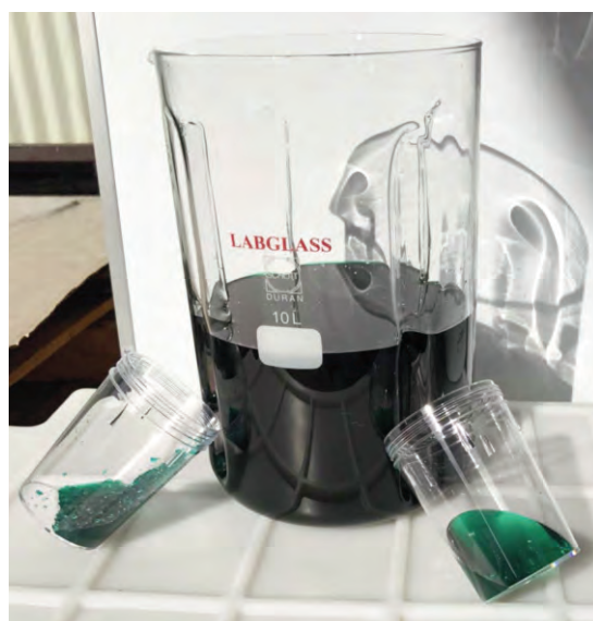
Figure 5: High purity Nickel Sulphate electrolyte generated from The DSX pilot plant
